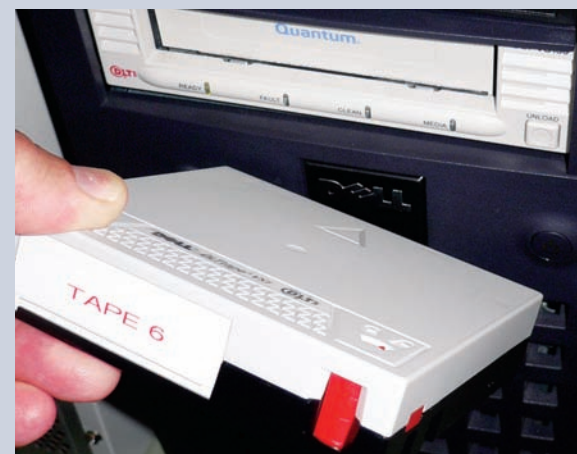
Figure 3. The security of digital images can be ensured by backing up data on the Internet, tape, or hard drives for off site storage. This tape can backup 80 GB and can be stored offsite for added security.
